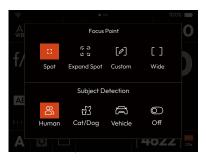
Tap the touch display or use the rear scroll wheel or 5D joystick to select the focus point mode. The focus point of the corresponding mode will appear in Live View. In Wide mode, the focus point will appear only when focus is correctly set.
