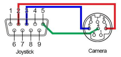
Serial/Analog RS-485 Control: To control your camera(s) over an RS-485 connection, see below.
