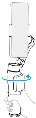
① Rotate the handle in the horizontal plane and the phone follows
