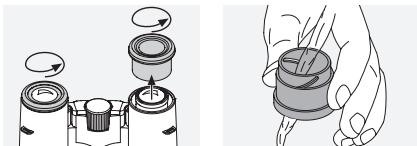
In the event of hard-to-remove dirt (e.g. sand) the eye cups can be unscrewed and cleaned easily.
