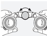
It is possible to bring every subject into focus from the shortest adjustment distance (see technical data sheet) to infinity by turning the focusing wheel.
