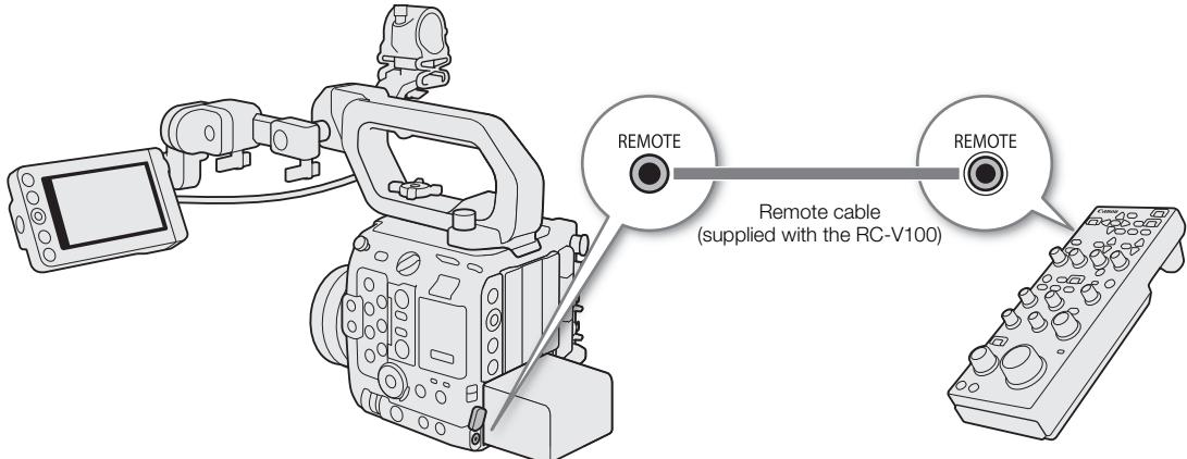
1 Turn off the camera and connect the optional RC-V100 Remote Controller to the camera.
