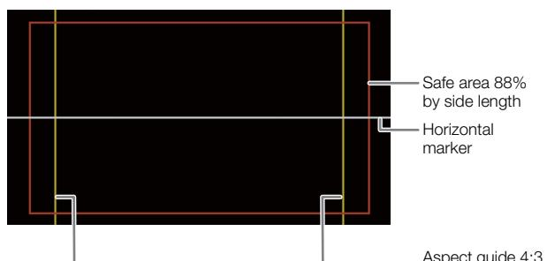
1 To display the markers overlay on individual video outputs, select **MENU** > [
