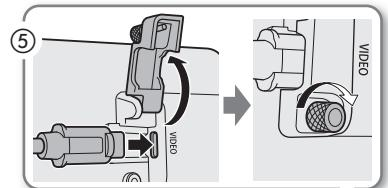
5 Put the cable through the handle unit's cable clamp (⑥).
