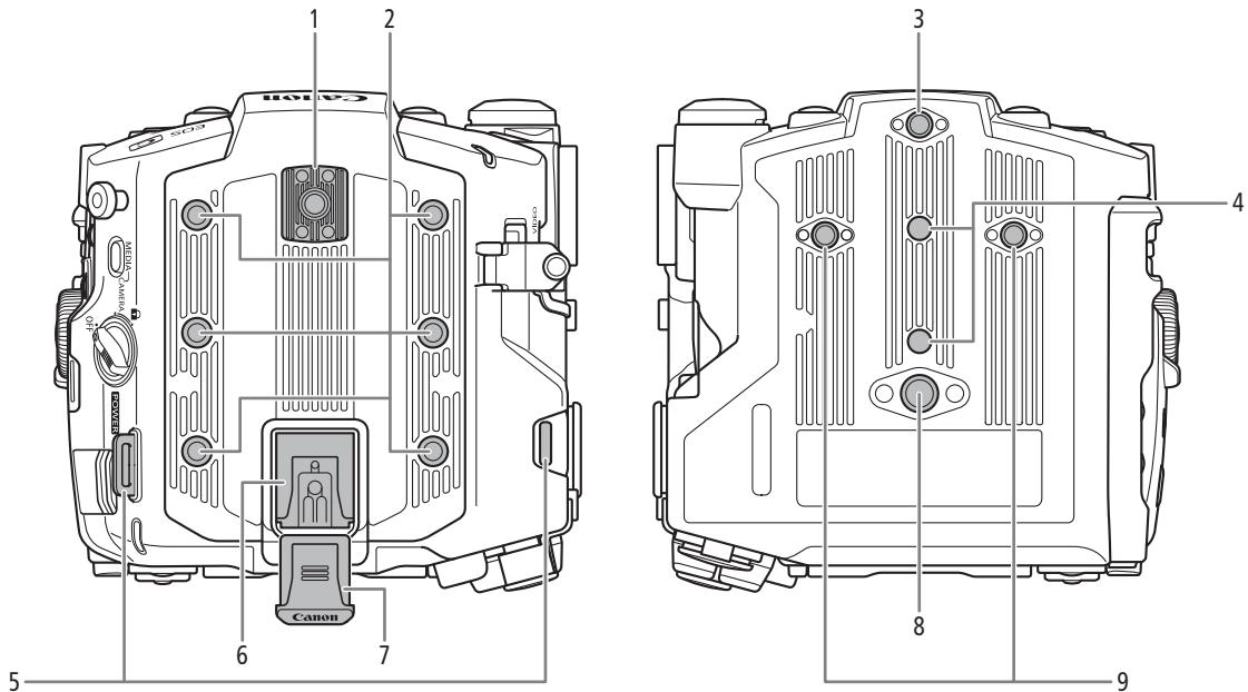
1 Accessory mount with socket for 1/4"-20 mounting screws (6.9 mm (0.27 in.) deep) (図 30)
