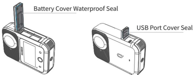
3. Before use, ensure the battery cover and USB port cover are fully locked (the latch must be completely engaged), otherwise the camera will not be waterproof.
